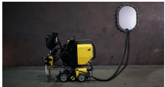
Modular design for hard to reach places. Min manhole 580 x 400 mm (23 x 16 in.) or circular hole of Ø 500 mm (20 in.)
